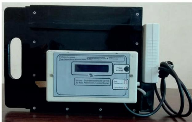
**Fig. 3.4.1. Moisture meter for raw cashewnuts, unpeeled and peeled cashew kernels**
