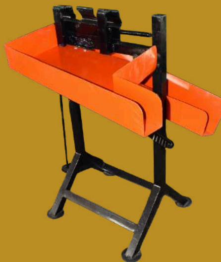
Fig. 3. Pedal-operated cashew apple and nut separator
