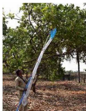
a) Battery Operated Telescopic Cashew Fruit Harvester
