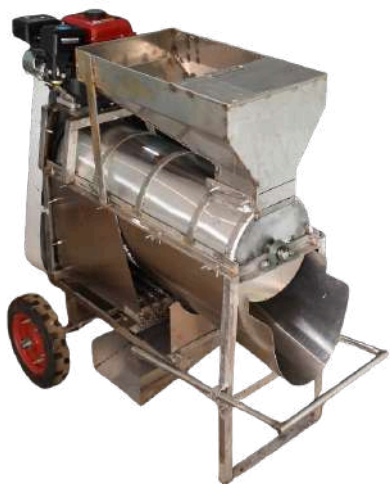
Fig. 5. 3-in-1 cashew nut separator, juice & pulp extractor, and fibrous material separator
