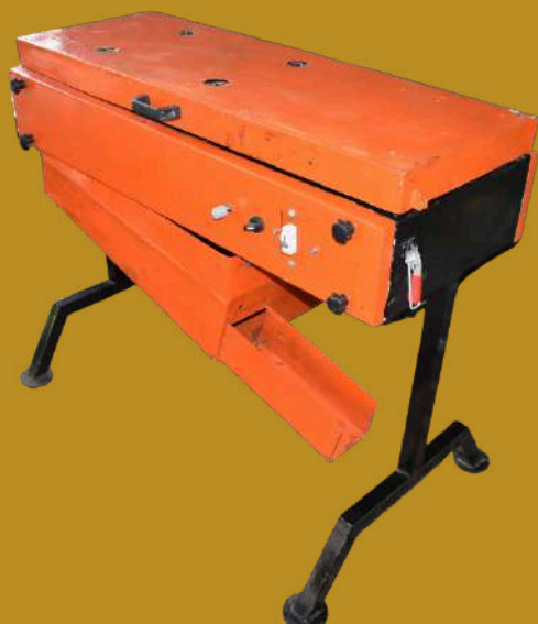
Fig. 4. Portable semi-automatic cashew apple and nut separator
